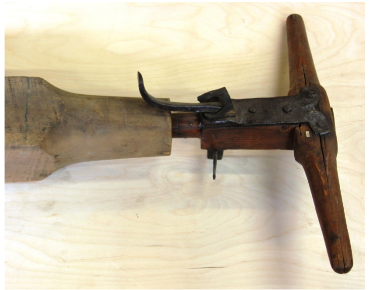
Two tools for cutting the male end of a pump log. "Turk's Head" to the left.
