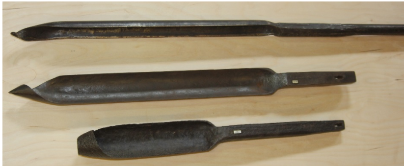
Upper – pod end of a 10' 6" hand auger Middle - replaceable bit for a hand auger Lower – replaceable reamer for a hand auger
