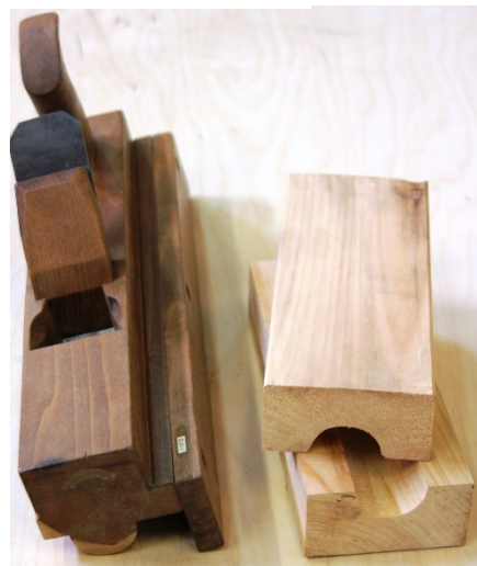
Two tools for cutting the male end of a pump log. "Turk's Head" to the left.
