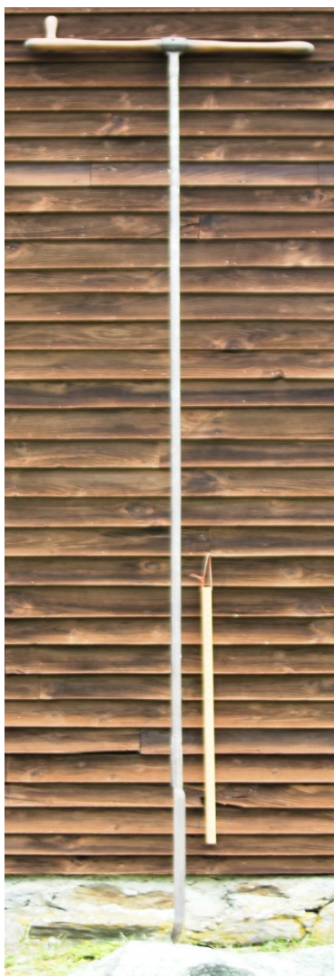
A 10' 6" manual pump log auger: a yard stick is shown for comparison.
