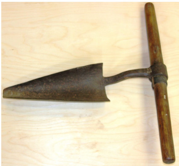
Reamer for cutting the female end of a pump log
