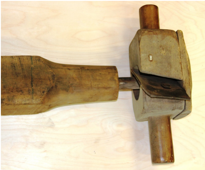
Two tools for cutting the male end of a pump log. "Turk's Head" to the left.
