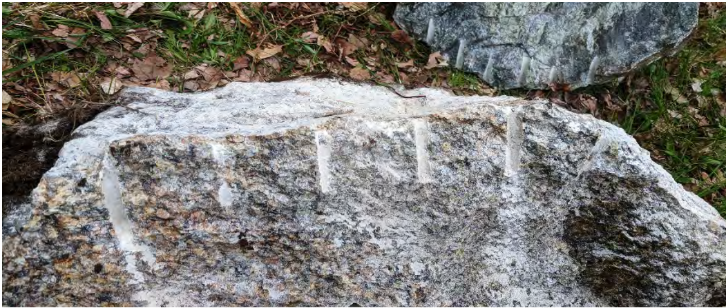
Face of rock above after splitting.
