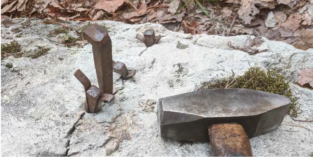
Feathers & wedges with spreading wedge in cracked schist boulder.
